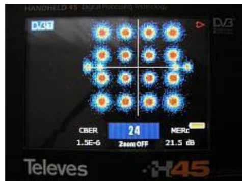
Picture 28 Constellation diagram, CBER a MERc 24 Ch.
