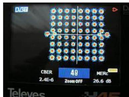
Picture 26 Constellation diagram, CBER a MERc 49 Ch.
