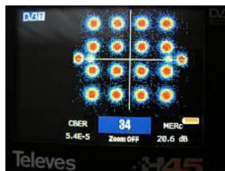
Picture 30 Constellation diagram, CBER a MERc 34 Ch.
