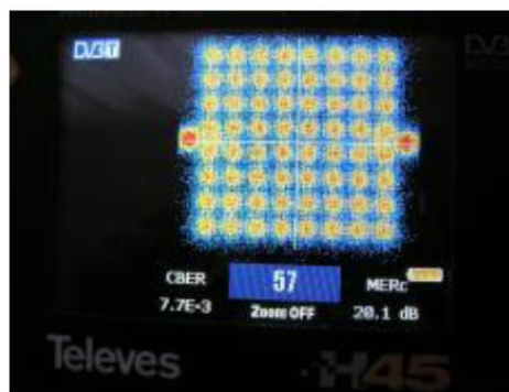
Picture 4 Constellation diagram, CBER a MERc 57 Ch.
