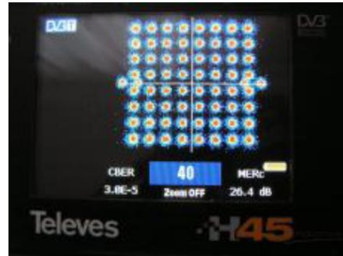
Picture 14 Constellation diagram, CBER a MERc 40 Ch.
