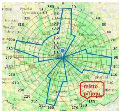
Picture 13 The signal covering – Brno-Kojál, 40 Ch.
