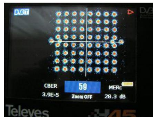
Picture 16 Constellation diagram, CBER a MERc 59 Ch.
