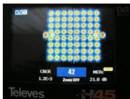
Picture 18 Constellation diagram, CBER a MERc 42 Ch.
