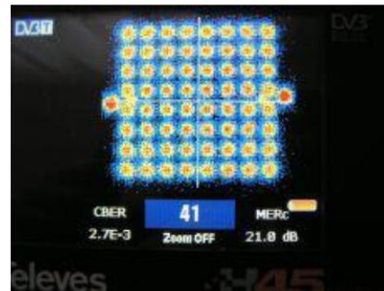
Picture 22 Constellation diagram, CBER a MERc 41 Ch.
