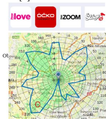
Picture 23 The signal covering – Zlín TI. hora, 25 Ch.
