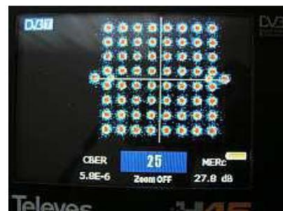
Picture 24 Constellation diagram, CBER a MERc 25 Ch.
