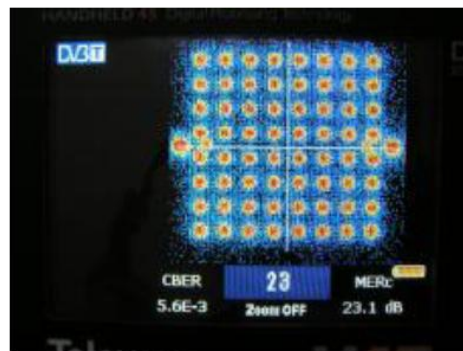
Picture 2 Constellation diagram, CBER a MERc 23 Ch.
