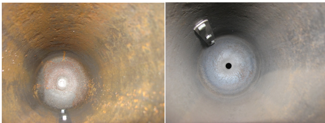
Figure 5 - The inside surface of the gas cylinder V = 10 l, D = 140 mm, L = 900 mm before and after cleaning using the proposed method
