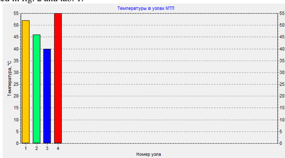
Fig 2. Integral temperature data acquired with ASONICA-P
