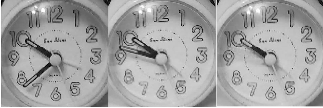
Fig. 1. The selection of the background (the scale indicator): a, b - image with different positions of the arrows; in the background is selected by taking the maximum of a and b.
