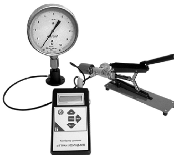
Figure 4 - Portable pressure calibrator Metran-502-PKD-10P
